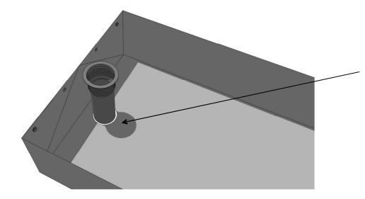
First, unscrew the lock nut & insert the threaded tube inside the drainage hole
