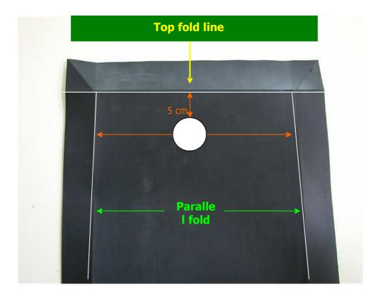
The hole should be made in the center, between the 2 fold lines (exp: 6.5-90-6.5 – The center would be 90 and the hole should be at 45cm from each side)
