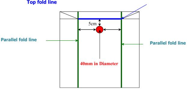
The diameter of the hole should be 40mm in diameter. **Top fold line**
