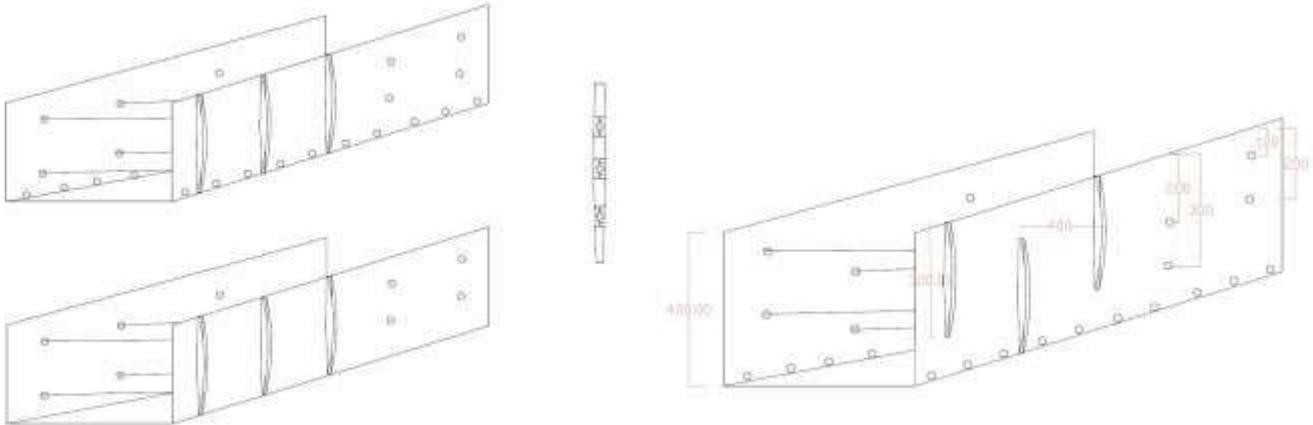
**Mapal troughs with drainage collection envelope plus spacer between the layers**
